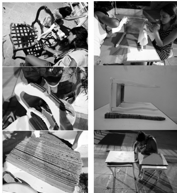
Figure 3. Cleaning, Painting and Production of the Missing Parts (left) Figure 4. Reproduction of the Side Table with Cardboard Sections (right)
