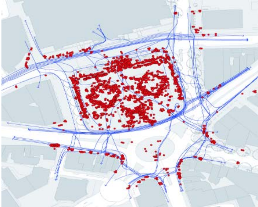
Figure 2. Motion analysis of Trafalgar Square with Space Syntax Method
