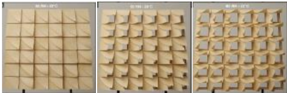
Figure 17. Reichert, Menges and Correa (2015), design of building material that moves depending on humidity and temperature
